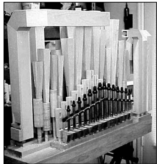
Figure 27. The completed windchest with all of the pipes installed.
