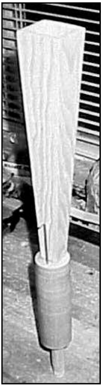
Figure 15. The wooden trumpet pipe.
