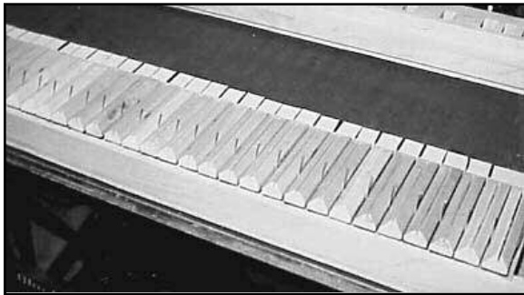
Figure 5. The pallet valves installed in the wind chest.
