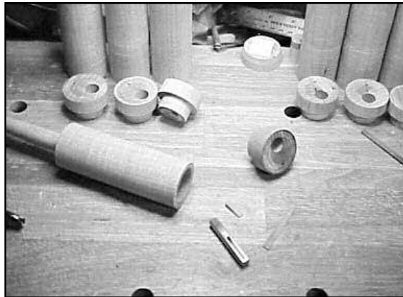
Figure 16. Components of the trumpet pipe.
