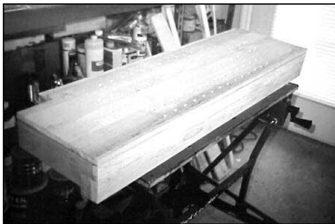
Figure 2. The windchest before adding risers for the pipes.
